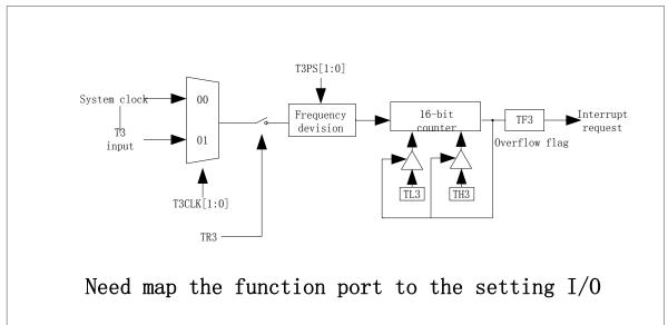
Figure 9 - 5 Timer3 function block diagram
