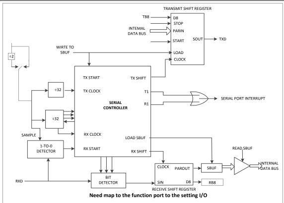
Figure 13 - 7 UART mode2 functional block diagram
