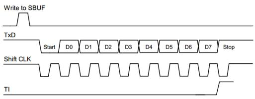
Figure 13 - 5 mode1 send the data time series block diagram
