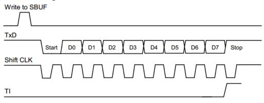
Figure 13 - 11 Send timing of mode0
