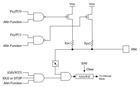
Figure 15 - 2 ADC power saving wakeup function block diagram
