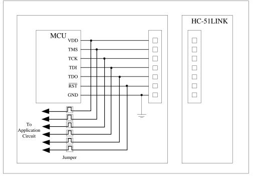
Figure 3 - 1 HC-51LINK programming hardware connection
