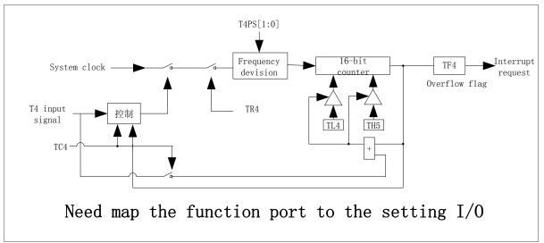
Figure 9 - 7 Timer4 mode2/3 functional block diagram
