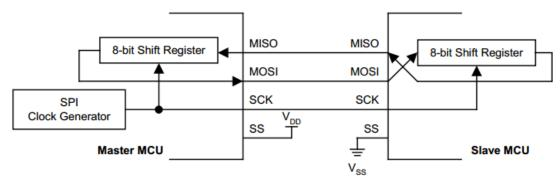
Figure 14 - 2 Full-duplex master/slave interconnect diagram
