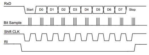
Figure 13 - 6 mode1 data receive timing diagram
