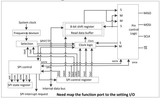
Figure 14 - 1 SPI functional block diagram
