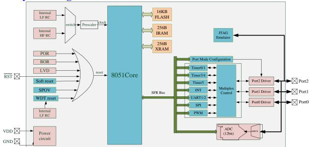
Figure 1-1 System diagram
