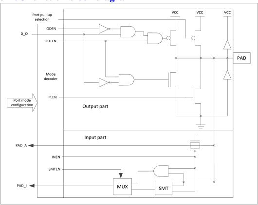
Figure 7 - 1 I/O function block diagram
