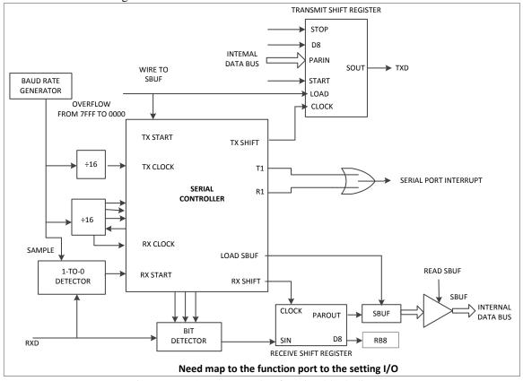
Figure 13 - 10 UART mode3 function block diagram
