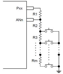
Figure 15 - 3 ADC series resistor key input application reference circuit
