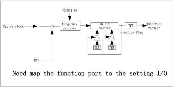
Figure 9 - 8 Timer5 Mode0 functional block diagram
