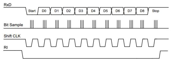
Figure 13 - 14 Receive timing of mode1
