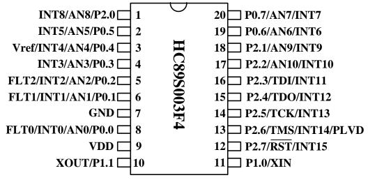
Figure 1-2 SOP20/TSSOP20 pin configuration diagram
