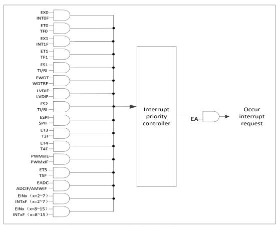
Figure 8-1 Interrupt function block diagram
