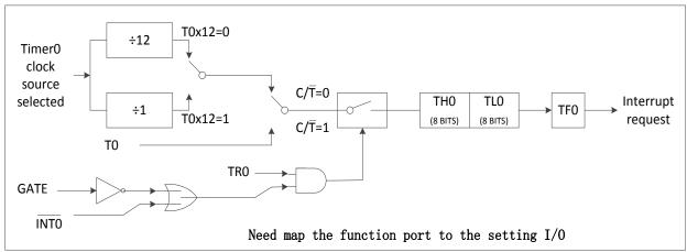
Figure 9 - 2 Timer0 1 mode1 function block diagram
