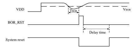
Figure 6 - 1 BOR schematic diagram
