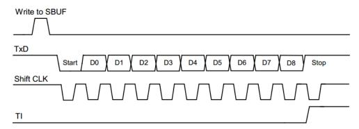
Figure 13 - 8 Mode2 Send the data time series block diagram
