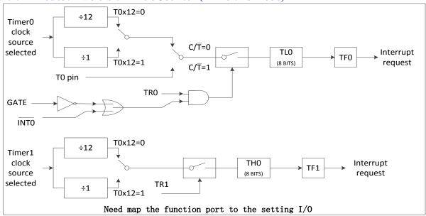
Figure 9 - 4 Timer0 3 function block diagram
