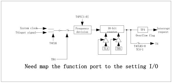
Figure 9 - 6 TIMER4 0 functional block diagram
