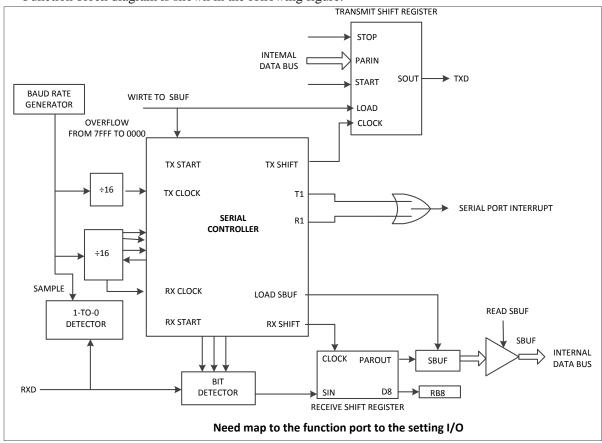
Figure 13 - 4 UART mode1 functional block diagram
