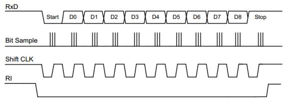
Figure 13 - 9 Mode2 receive data timing diagram
