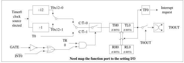
Figure 9 - 1 Timer0 mode0 function block diagram
