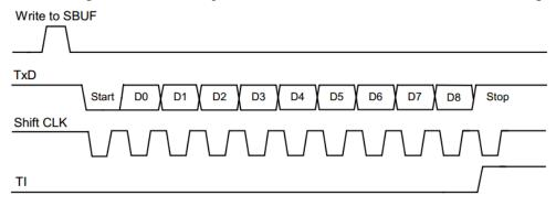
Figure 13 - 13 Send Timing of mode1
