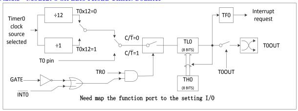
Figure 9 - 3 Timer0 mode2 Function block diagram
