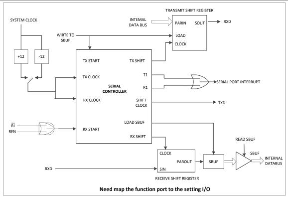
Figure 13 - 1 UART mode0 function block diagram
