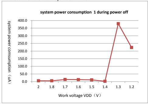
Figure 19 - 1 system power consumption 1 during power off
