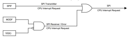
Figure 14 - 6 SPI interrupt request generation
