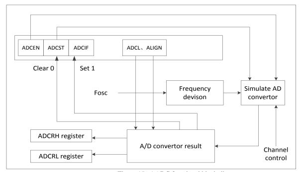
Figure 15 - 1 ADC functional block diagram
