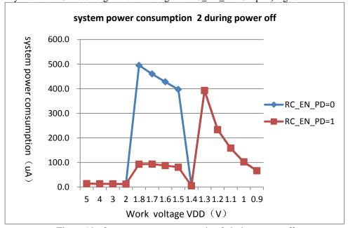
Figure 19 - 2 system power consumption 2 during power off
