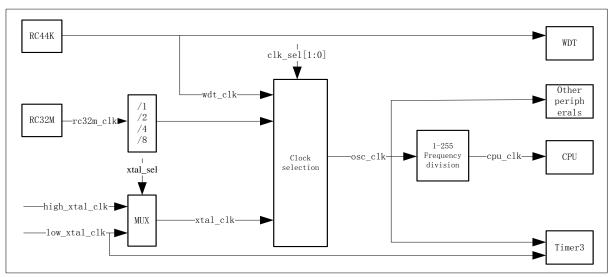
Figure 4 - 1 System clock block diagram
