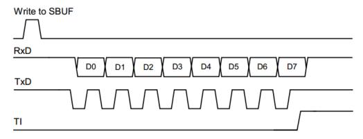
Figure 13 - 2 Mode0 data send timing diagram
