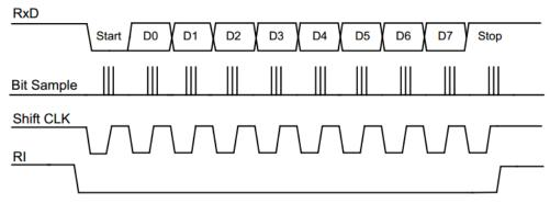
Figure 13 - 12 Receive timing of mode0
