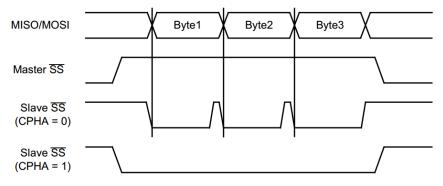
Figure 14 - 5 CPHA/ $(\overline{SS})$  timing sequence
