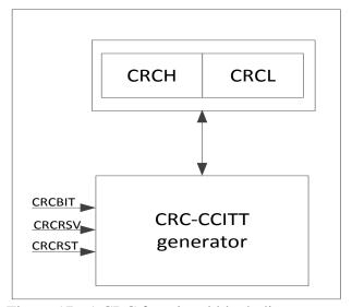
Figure 17 - 1 CRC functional block diagram
