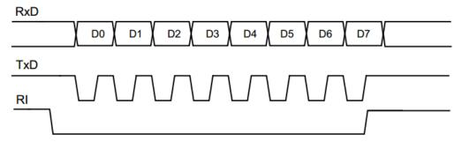
Figure 13 - 3 Mode0 Data receive timing diagram
