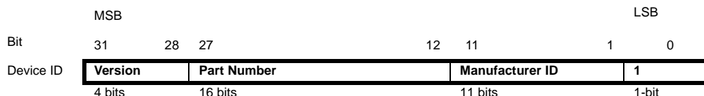
Figure 27-1. The Format of the Device Identification Register
