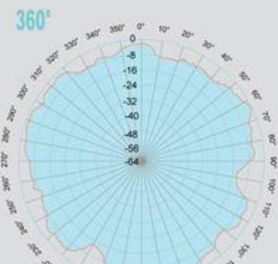
PD-V3 360° 5.8GHz Microwave Motion Sensor is a C-Band Bi-Static Doppler transceiver module. It adopts built-in Resonator Oscillator (RCO) amplified signal external circuit. More sensitive and lower power consumption than V2. It is convenient for the customers to develop various products.
