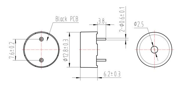
\*Unit: mm; Tolerance: ± 0.5mm Except Specified
